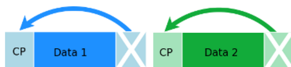
Figure 2.1: OFDM Symbols with Cyclic Prefix
