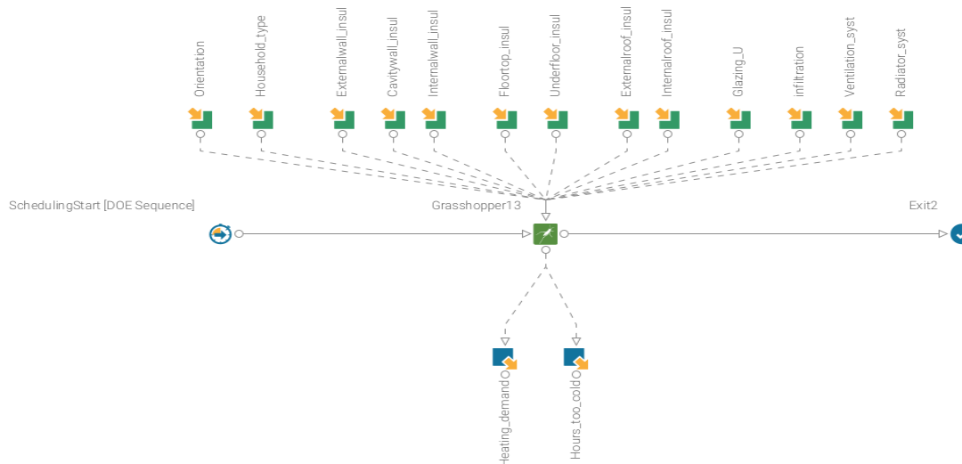
Figure 29 - modefrontier workflow and input-output parameter overview
