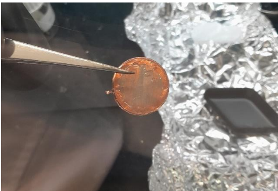
Figure S 9. Onset plating of lithium after 2 hours of plating at 0.1 mA/cm 2 with 100mM BTATFSI in 1 M LiPF 6 in 1:1:1 EC:DMC:DEC in a Li:Cu cell.
