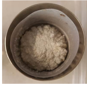
Figure 4.15: Ni crucible used in NaOH conversion process after conversion
