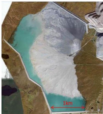
Figure 3.1: Satellite photo of the tailings pond at the LKAB mine at Kiruna (picture courtesy of the REEcover project)
