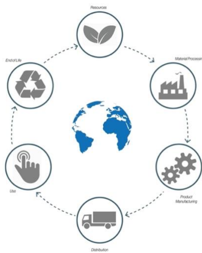
Figure 4 Cradle-to-grave stages used in LCA
