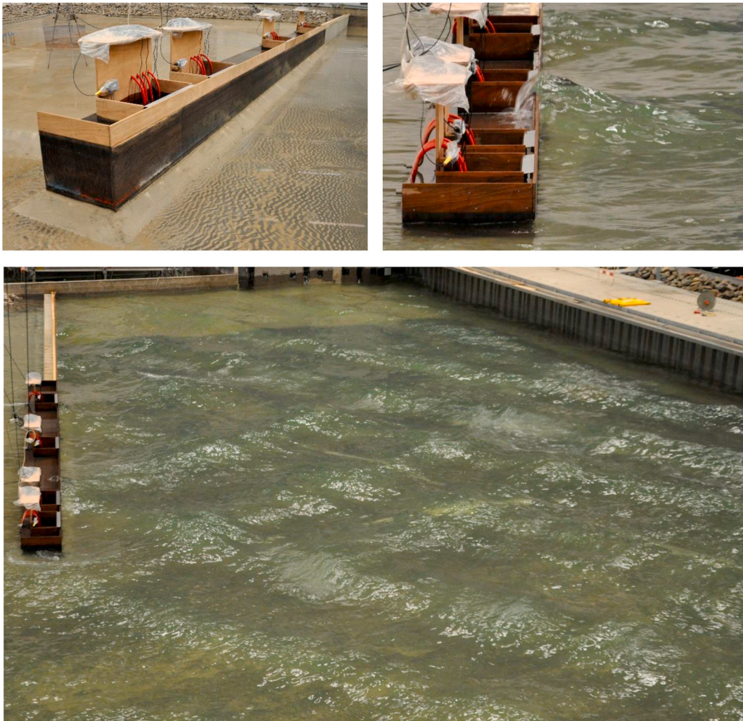
Fig. 7. View of the model in the dry wave basin in the upper-left panel, an overtopping event in the upper-right panel, overviews of the model in the wave basin in the next two panels with the wave pattern of incident and reflected waves (clapotis gauffré), and images of overtopping events in the lowest two panels.
