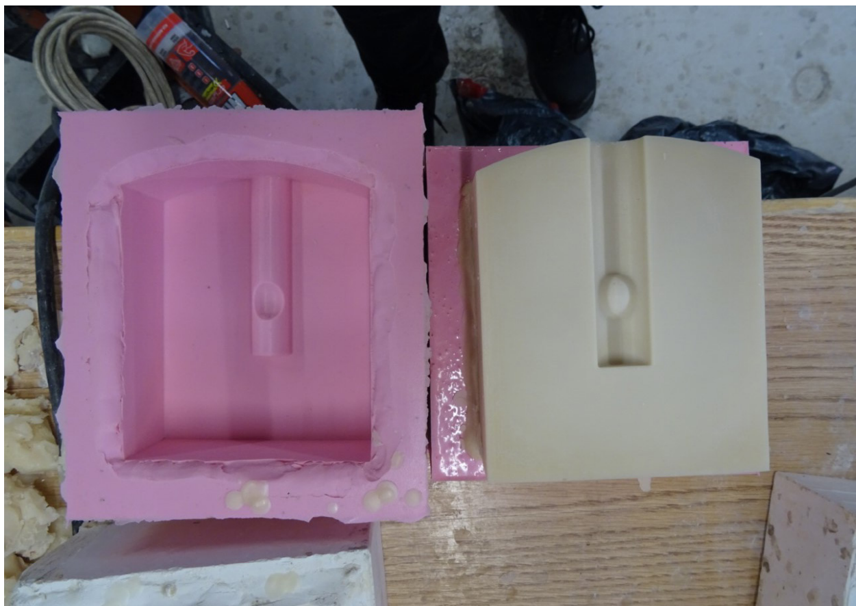
Figure 5.4 From 3D printed model, to silicon mould, to wax model
