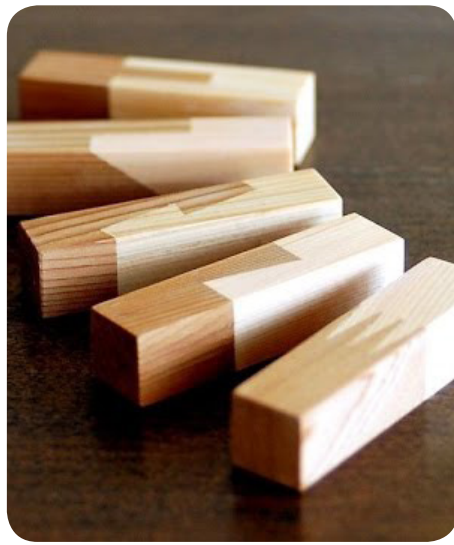
Figure 3.5 Japanese wood connections
