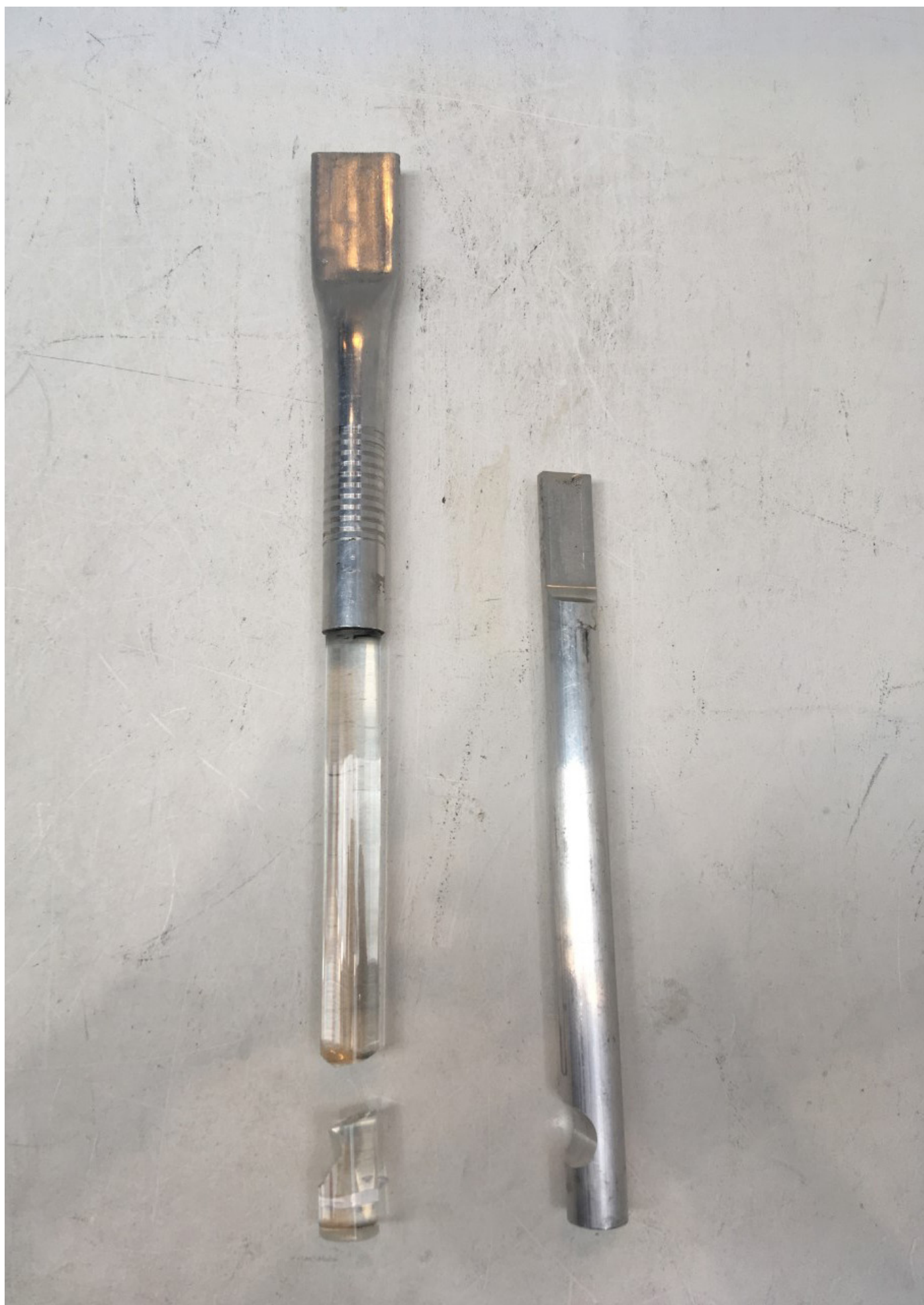
Figure 5.29 From aluminum plus glass connection piece to an all aluminum one
