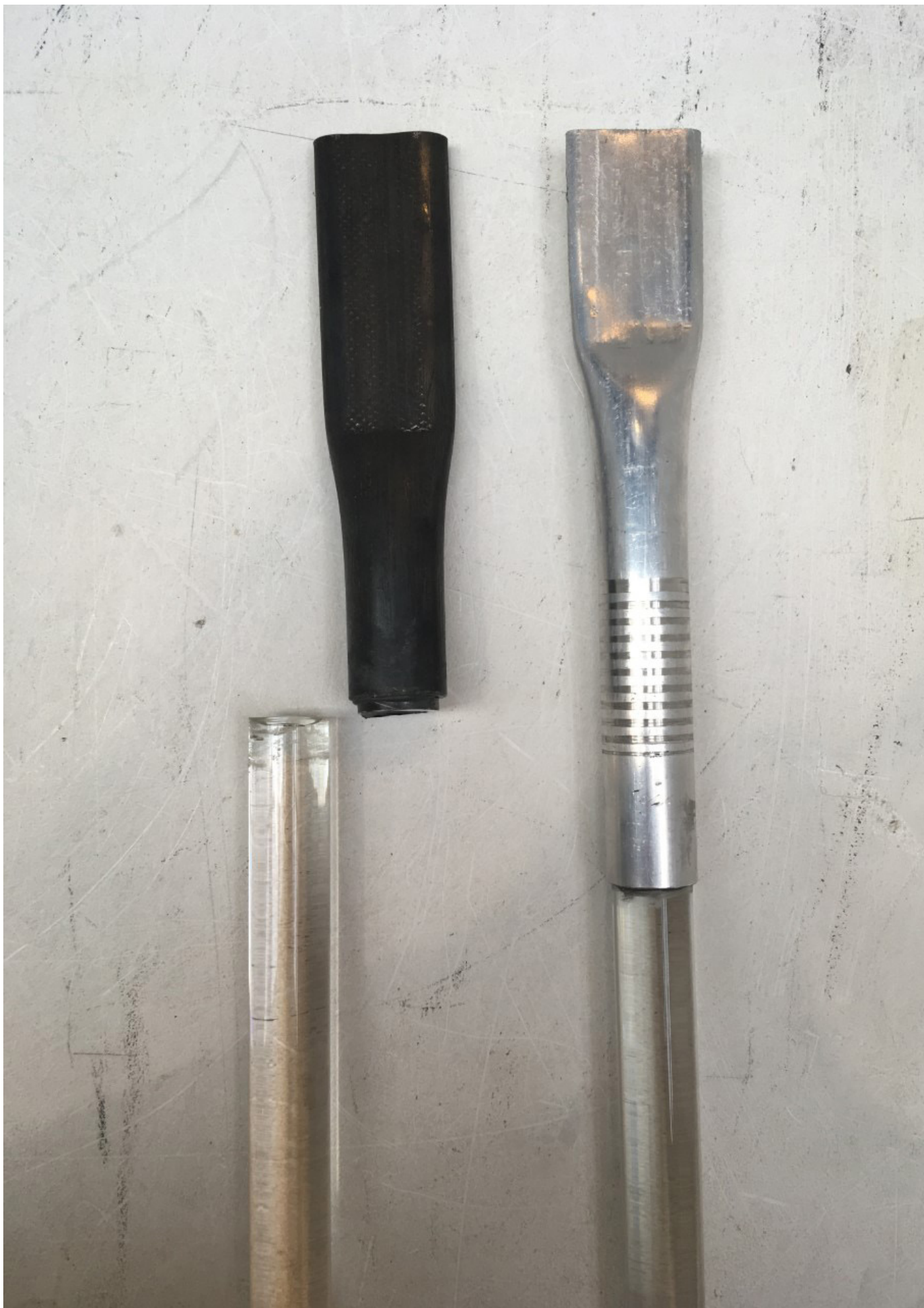
Figure 5.26 From steel connection piece to an aluminum one
