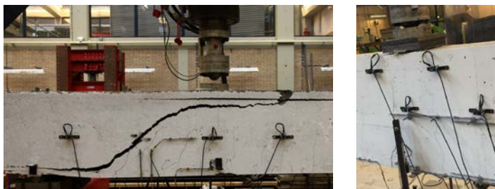
Fig. 1 Left: Beam RSB03A after shear failure. Right: Beam P804A1 after flexural failure.
