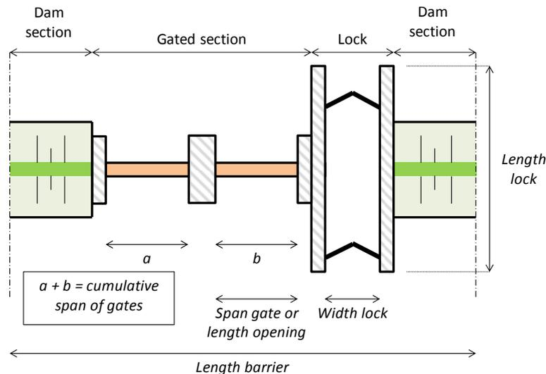
Figure 1: Basic top view of a storm surge barrier
