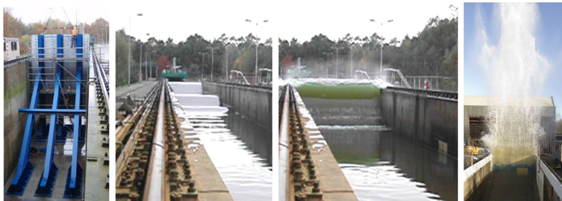
Figure 2.2 Large scale wave impacts at vertical walls in the Delta flume, Deltares, Hofland et al. 2010. Left panel: Lee side of vertical wall, Mid panels: Wave propagation and breaking, Right panel: Wave impact at the vertical wall.
