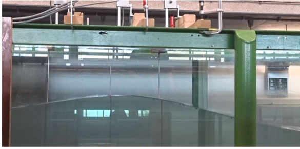
Figure B2.3. Photo sequence from focused wave test E004 at the offshore measurement location, target focal point, x_f = 24.7 m, incident wave height, h_i = 0.237 m measured at gauge G15.
