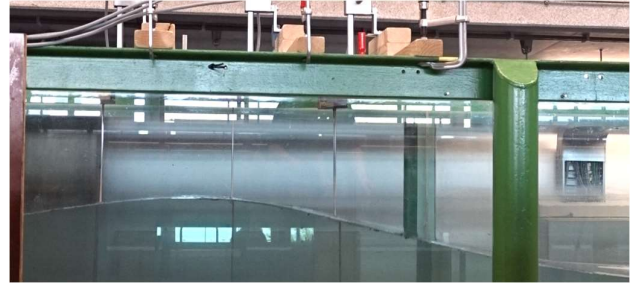
Figure B2.3. Photo sequence from focused wave test E004 at the offshore measurement location, target focal point, x_f = 24.7 m, incident wave height, h_i = 0.237 m measured at gauge G15.
