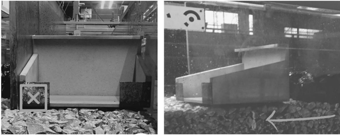
Figure 4.13 Model crest wall. Left panel indicates the metal plate where the proximity switch aimed to measure the displacement. Right panel indicates the displacement direction. Note this core material does not represent the one tested in these experiments.
