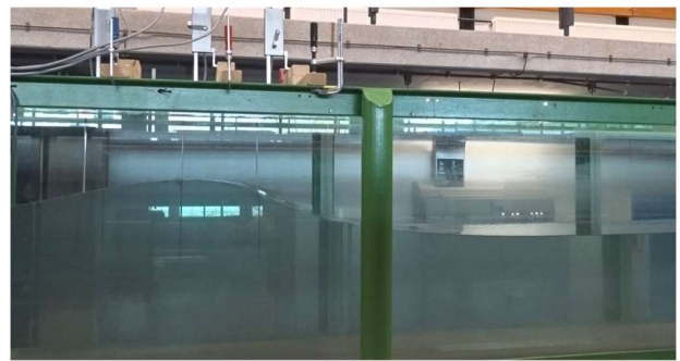
Figure B2.4 Photos during focused wave test E007 at the offshore measurement location, target focal point: x_f = 26.70 m, incident wave height, H_i = 0.238 m measured at gauge G15.
