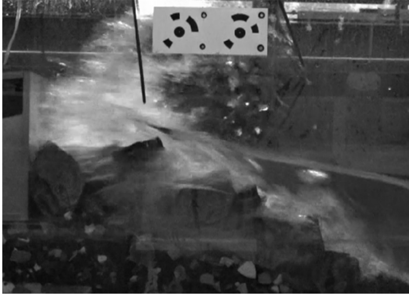
Figure 4.2 Close up wave impact at the crest wall during a focused wave test.
