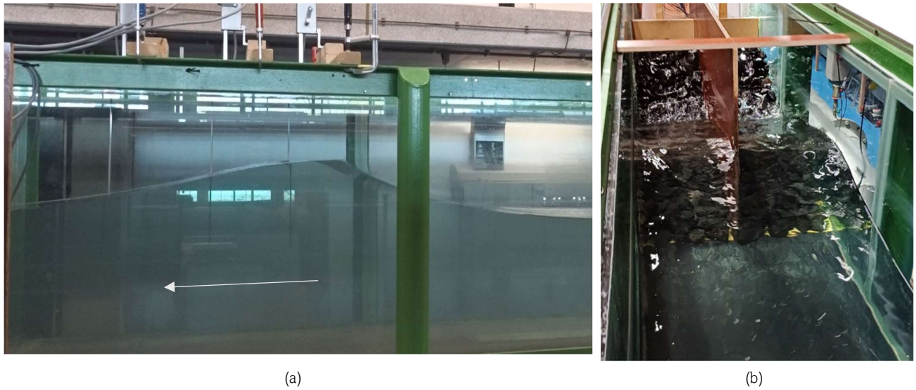
Figure 3.2 Wave propagation in the flume. (a): Side view of the flume while focused wave propagates at the offshore measurement location. Arrow is pointing the propagation direction. (b): Front view of the testing section during irregular wave tests prior to a wave impacting the slope.
