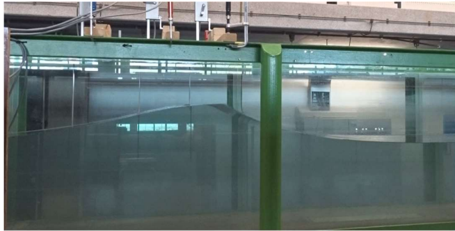
Figure B2.4 Photos during focused wave test E007 at the offshore measurement location, target focal point: x_f = 26.70 m, incident wave height, H_i = 0.238 m measured at gauge G15.
