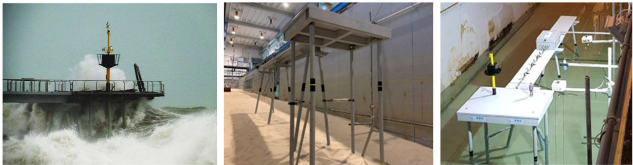
Figure 2.3 Left panel: Wave attack at pier, at Pont del Petroli during storm Gloria, source: Badalona City Council, Spain, Middle and Right panel: physical model tests at CIEM flume, at UPC, Spain, Altomare et al (2024, b).
