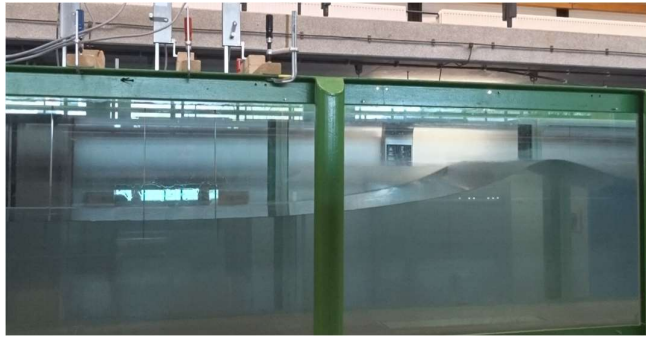
Figure B2.3. Photo sequence from focused wave test E004 at the offshore measurement location, target focal point, x_f = 24.7 m, incident wave height, h_i = 0.237 m measured at gauge G15.
