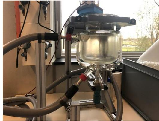
Figure A1 Crystallizer for the batch experiment
