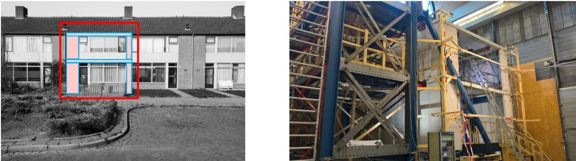
**Figure 2.2:** (a) Load bearing structure of Dutch terraced houses (Esposito et al., 2016) (b) Set-up experiment BUILD\_TUD-2 in Stevin lab 2 at TU Delft (Schippers, 2017).
