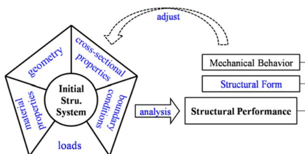
Figure 2: The conceptual scheme of numerical form-finding
