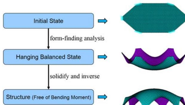
Figure 1: The basic procedure of the numerical method
