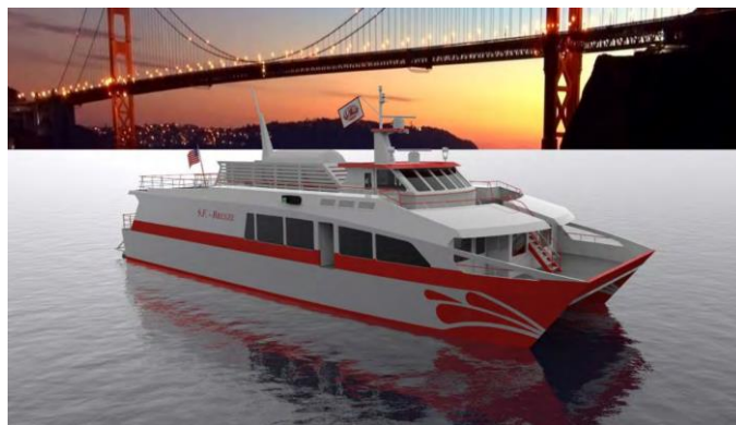
Figure 3.6: render of the SF-BREEZE, a hydrogen fuel cell powered ferry in the San Francisco Bay. [13]
