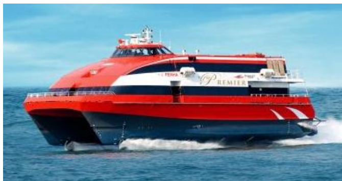
Figure 6.1: Foilcat, a hydrofoil catamaran, in fully foilborne condition. [102]
