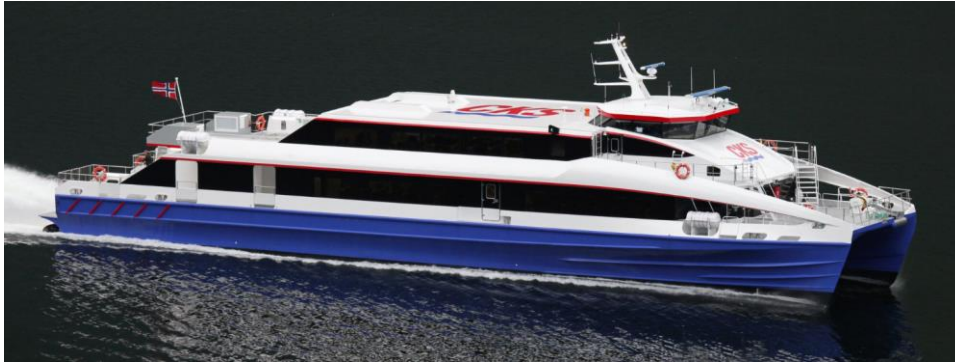
Figure 5.3: the Zhong Shan 6, a 44 m long carbon composite catamaran that can transport 300 passengers with a speed of 40 knots.
