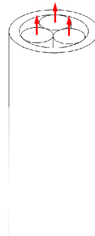
Figure 2.2: Conceptual design of a single cannula with a lumen containing multiple elements which allow up and down movement. The arrows represent the motion of the elements.
