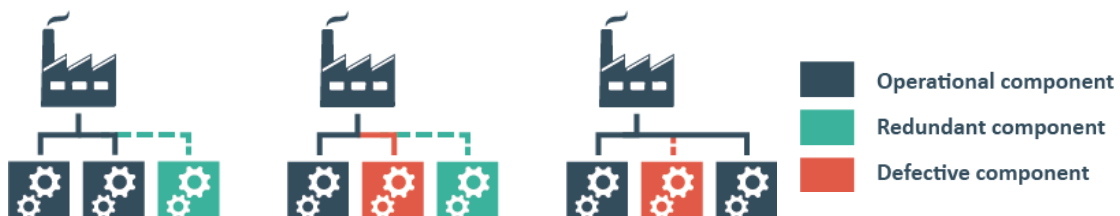
Figure 7: The concept of redundancy (own illustration)
