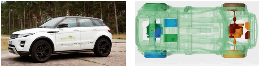
Fig. 1. SUV demonstrator with individual on-board motors.
