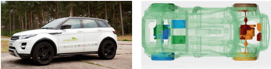
Fig. 1. SUV demonstrator with individual on-board motors.
