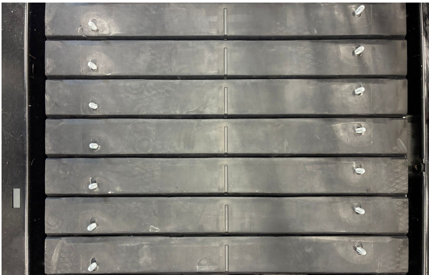
Figure 2.3: Top view of the Technogym Skill Run slatted belt, showing the individual rubber slats connected by a continuous loop.
