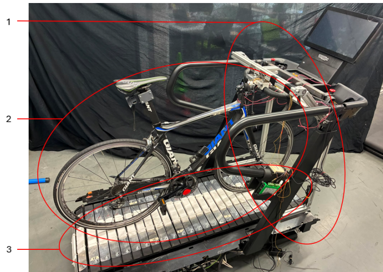
Figure 2.21: Photograph of the complete measurement apparatus, showing the bicycle (1), stabilization mechanism (1) and 3D printed road surface (3).
