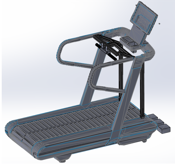
Figure 2.20: CAD representation of the treadmill with the stabilization mechanism. The bicycle is omitted for clarity; the black bar represents the handlebar at the connection point between the bicycle and the stabilization mechanism. The 3D printed road surface is not shown.
