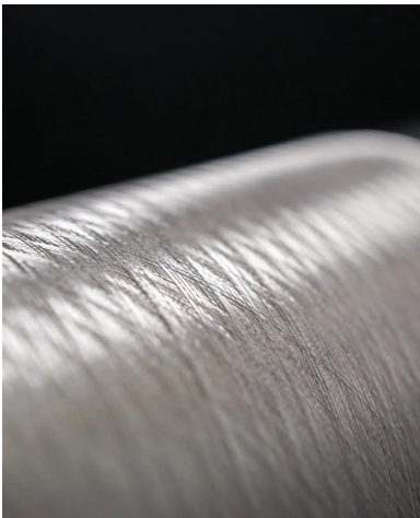
Figure 24.3 Spintex Engineering’s bio-based and biodegradable silk fibers are made at room temperature in non-toxic, water-based chemistry
