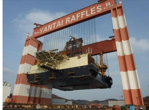
Figure 2-15 - Taisun gantry crane (cimc-raffles.com)
