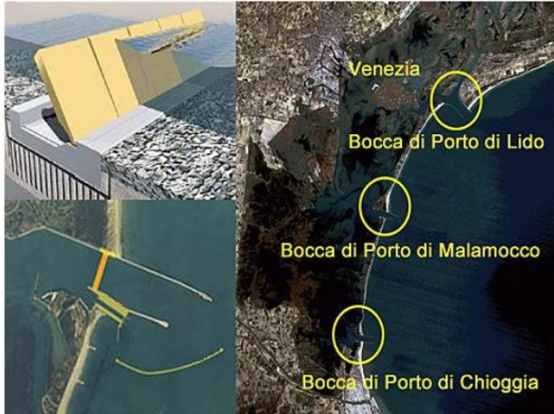
Figure A-17 - Type of flood defence, plan view of flood defence, location of immersing caissons (dutchwatersector.com, 2013)
