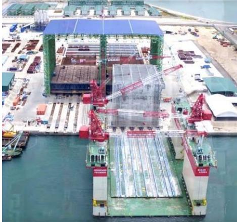
Figure A-5 - Transportation of caisson on semi-submersible vessel (Krabbendam, 2016)
