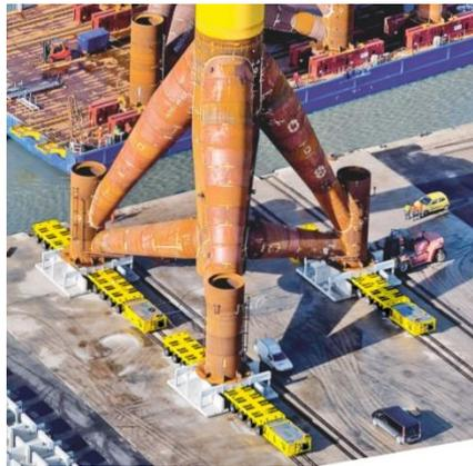
Figure 2-11 - SPMTs transporting a tripod foundation (scheuerle.com)
