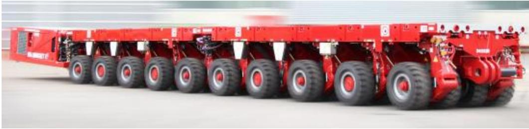
Figure 2-10 - Self Propelled Modular Transporter (scheuerle.com)
