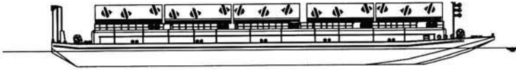
Double deck RoRo barge for 32 trailers (in service between Passau and Budapest since 1992) L_{oa} = 76.5 m, B = 11.4 m
