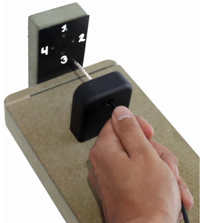
Figure 21: Close-up of the experimental setup. The four targets are indicated by a number. The secondary hand is placed in front of the insertion block to push and pull the shaft.
