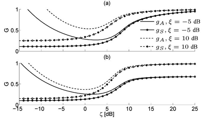
Fig. 2. Complex-DFT and DFT-magnitude gain curves for  $\xi = -5$  dB and  $\xi = 10$  dB, for (a)  $\gamma = 1, \nu = 0.6, K = 20$  and (b)  $\gamma = 2, \nu = 0.15$ .
