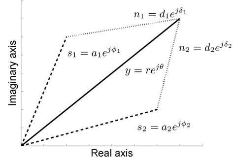
Fig. 1. Consider  $y$  which could result from many different speech and noise DFT-coefficient pairs, for example,  $s_1 + n_1$  or  $s_2 + n_2$ . Under Assumptions 1) and 3),  $f_{Y|S}(y|s)$  is given by (2) and depends only on the magnitude  $d = |y - s|$  of the noise DFT coefficient  $n$ . Therefore,  $f_{Y|S}(y|s_1)$  equals  $f_{Y|S}(y|s_2)$  when  $d_1 = d_2$ .
