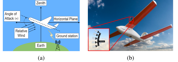
Fig. 1: (a) Angle of Attack (AoA) made by an aircraft. (b) Conceptual view of Hermes on a fixed-wing UAV.
