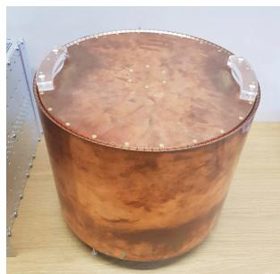
(a) Exterior of the low-field MRI prototype.
