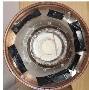
(b) Inside of the low-field MRI prototype.
