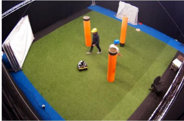
Figure 4.2: Dataset recording using the OptiTrack motion capture system. Two pedestrians are walking around wearing safety helmets fitted with reflective markers.
