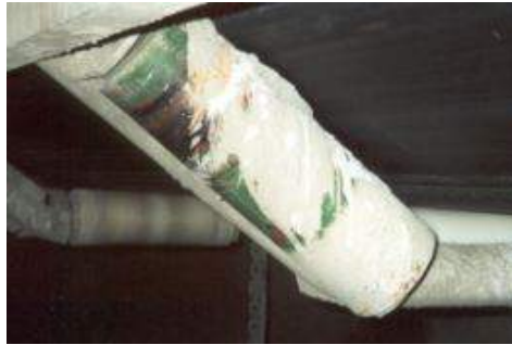
Figure 2.4: Build-up of materials on an idler roll, figure courtesy of Nylocomp Ltd.
