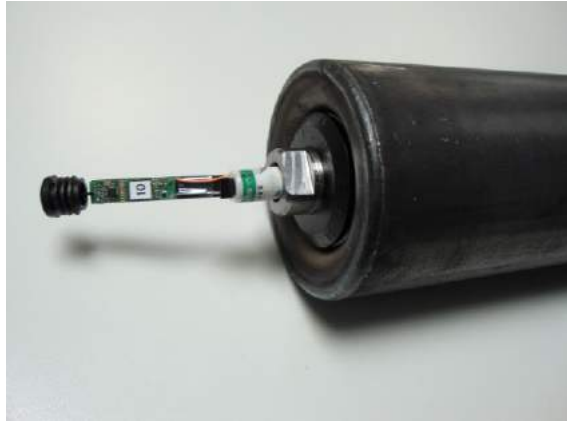
Figure 5.3: The "Smart Idler" at the RFID Laboratory of Delft University of Technology (Pang and Lodewijks, 2011).
