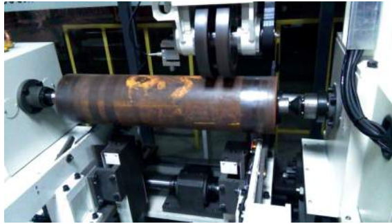
Figure 5.21: Idler roll rotating resistance measurement apparatus, figure courtesy of Rizhao Changyun Industry Transport Equipment Co., Ltd.
