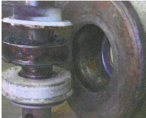
Figure 2.9: Contamination of rolling bearing, derived from Geesmann et al. (2008).
