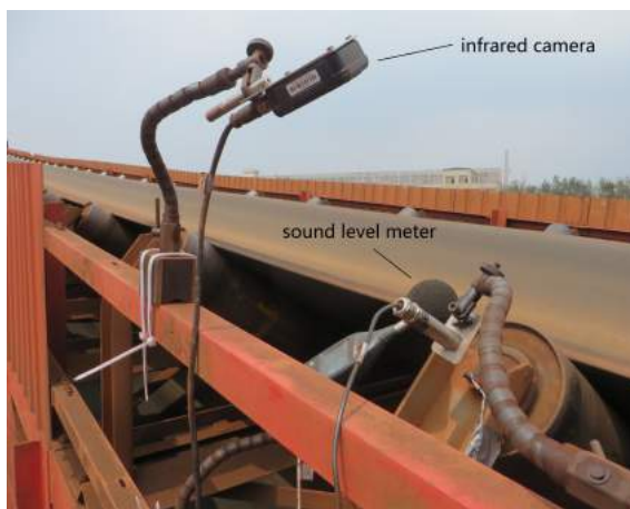
Figure 5.20: In-situ idler experimental setup.
