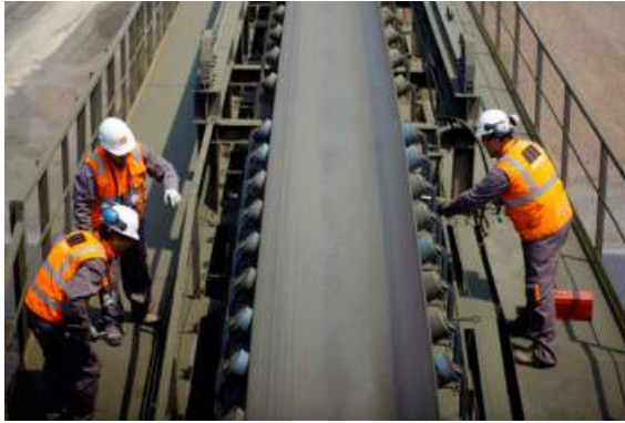
Figure 5.1: Manual inspection of belt conveyor idlers, figure courtesy of Martin Engineering (2014).
