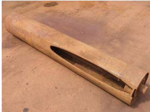
Figure 1.4: A typical failed idler roll, figure courtesy of Rizhao Port Group Co., Ltd.
