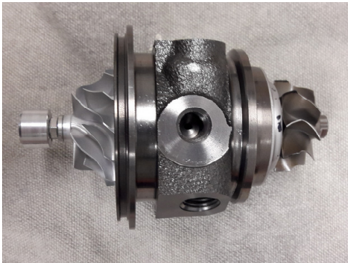
(a) Modified turbocharger rotor-bearing system: top view. The rotor features an additional cylindrical section in front of the compressor wheel (left hand side).
