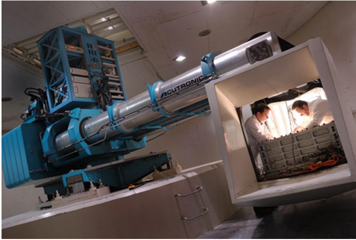
Figure 6.1 C-CORE's 5.5m-radius, 200g payload capacity Actidyn centrifuge (C-CORE, s.a.-d)
