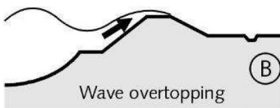
Figure 2.8 Failure mechanism: wave overtopping (Weijers & Tonneijck, 2009)
