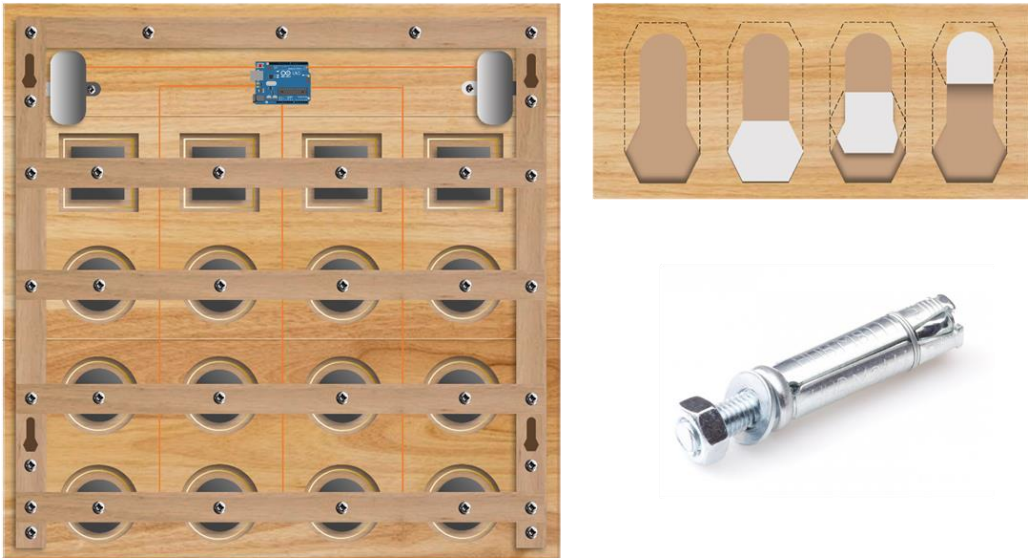
Figure 80. Holes for the toggle bolts in the suspension system (Techniek Webshop, n.d.)
