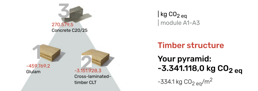
CARBON IN STRUCTURE
