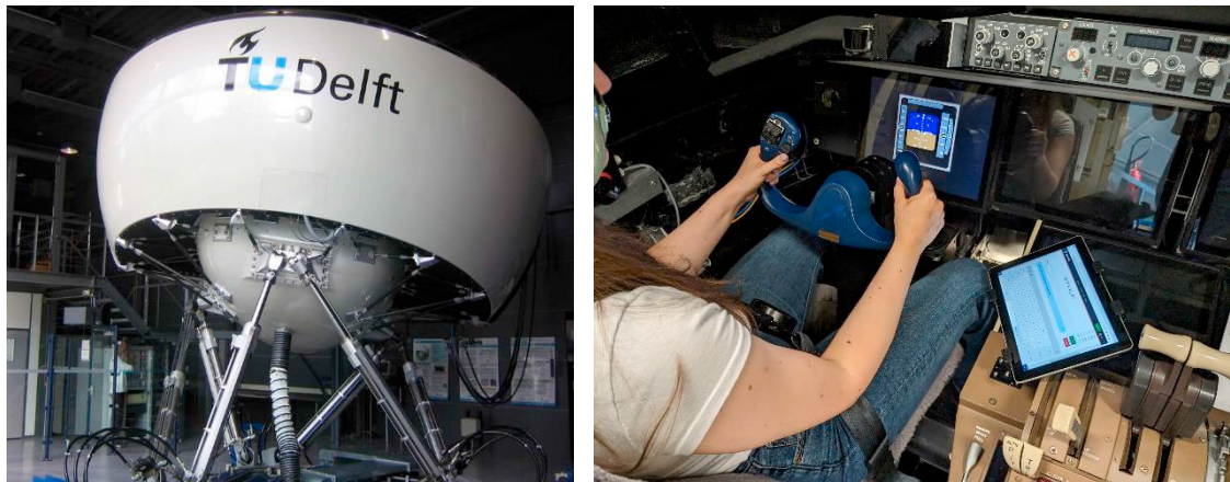
Fig. 2. The SIMONA Research Simulator (left) and the experimental setup (right).
