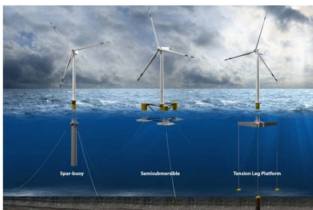
Figure 1.5: The three floater foundation concepts. Spar-buoy (Spar), Semi-submersible (Semi-Sub) and Tension Leg Platform (TLP) [28]
