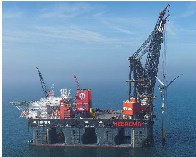
Figure 1.2: Heerema's Sleipnir installing the pilot 2.75 MW WTG for the FOX project, Courtesy of Heerema
