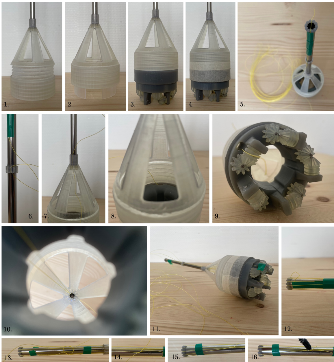
Figure 45: Snapshots made throughout the assembly of the device.
