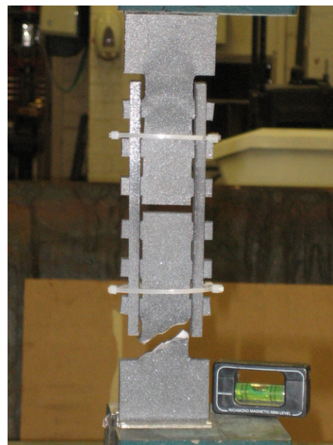
Figure 9. Failure mechanism of scaled side ISC flanges
