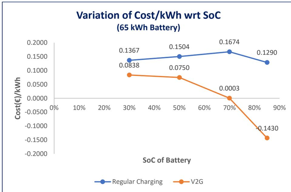
Figure 5.3 Variation of Cost/kWh w.r.t SoC
