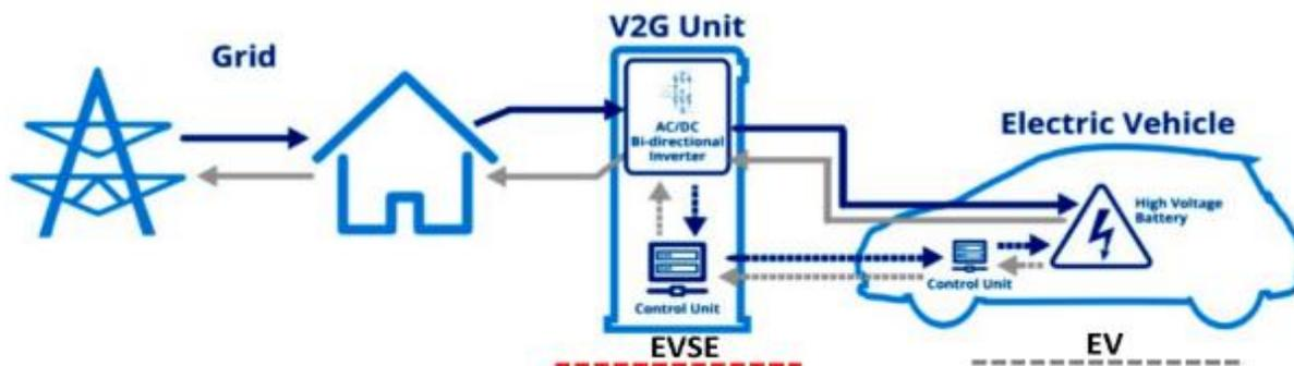
Figure 2.1 Vehicle-to-Grid System (Jaman et al., 2022)
