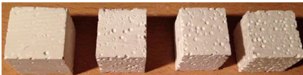
Fig. 1. Gypsum plaster specimens (about 20 × 20 × 20mm) with different amounts of porosity (measured from tomography images), left to right: 12.9%, 22.6%, 30.4%, and 30.0% [46].
