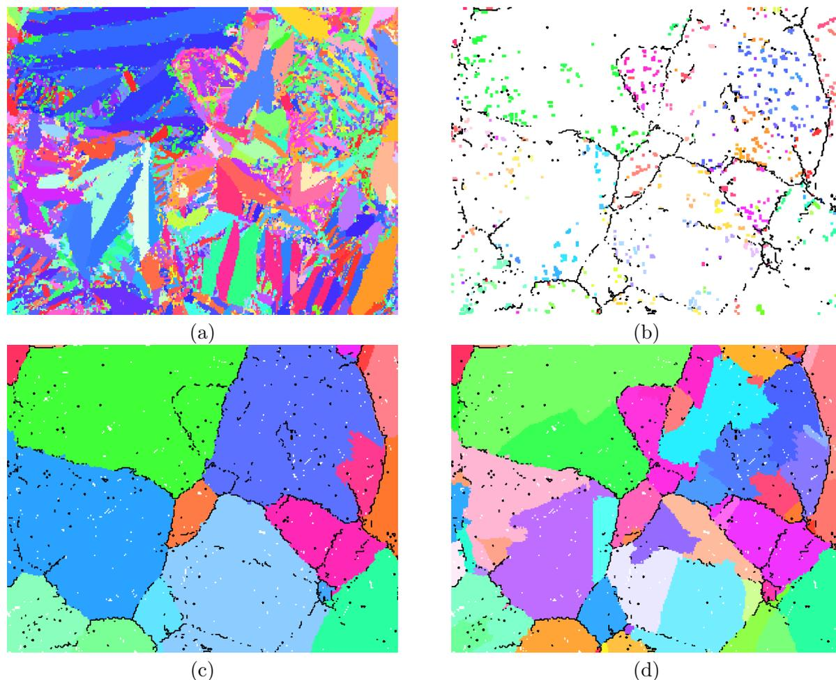
**Figure 3.** Validation of reconstruction algorithm on Fe-Ni alloy: (a) initial OIM before reconstruction, (b) retained austenite and expected prior austenite GB, (c) reconstruction after the first iteration and (d) second and final step of reconstruction.
