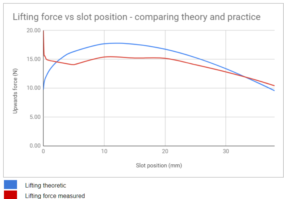
Figure A60: Lifting force vs slot position, theory and practice
