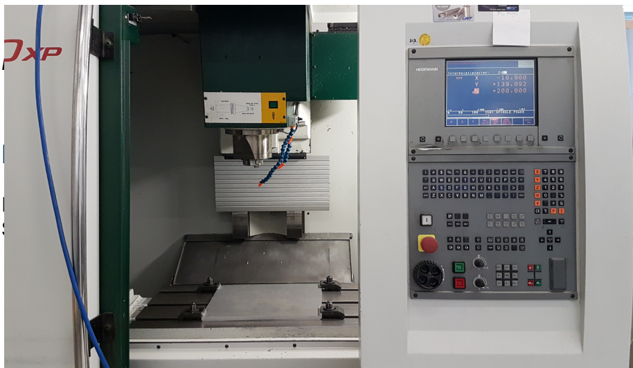
Figure A58: Aluminum plate in CNC machine
