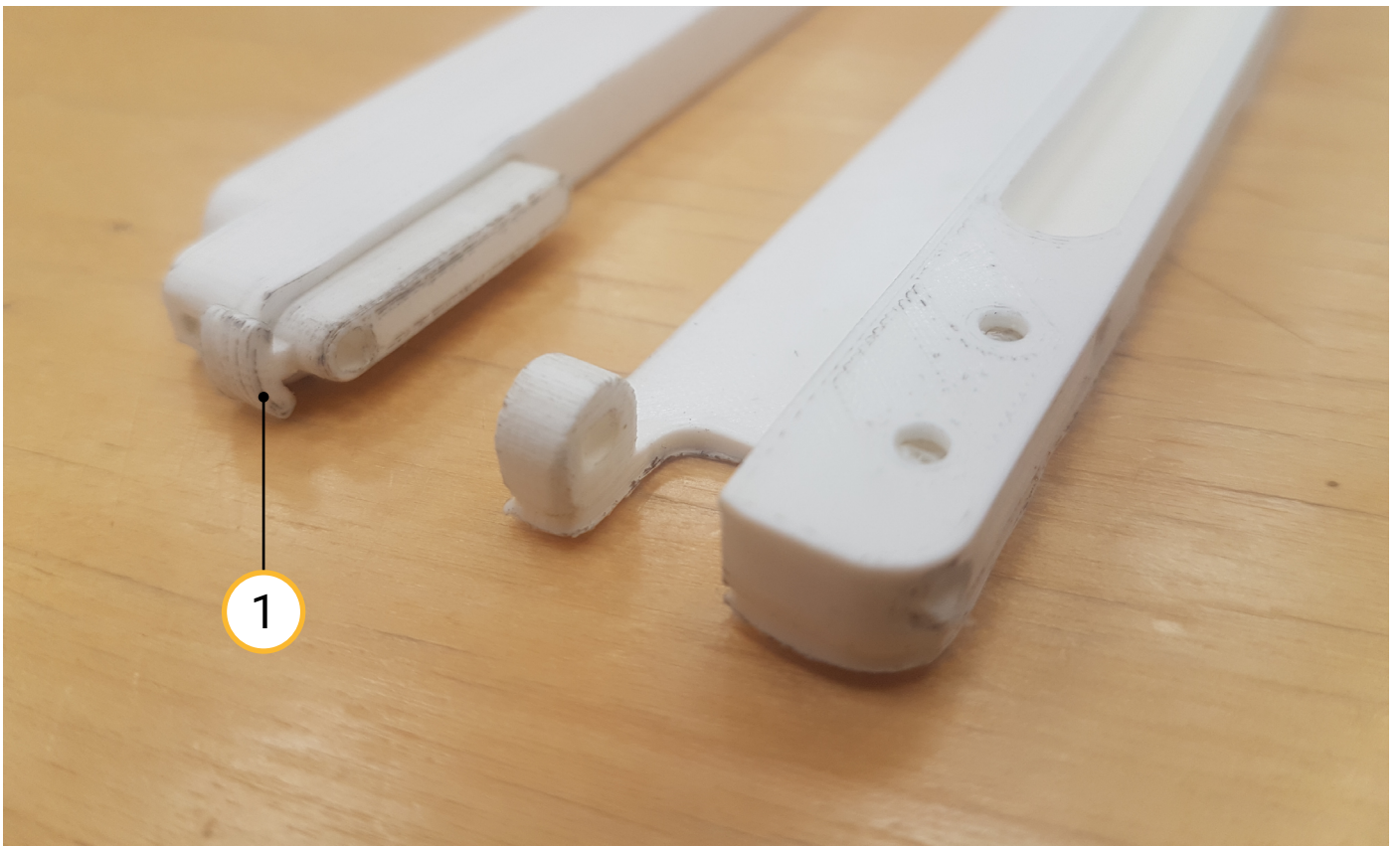
Figure A48: 3D print of locking mechanism
