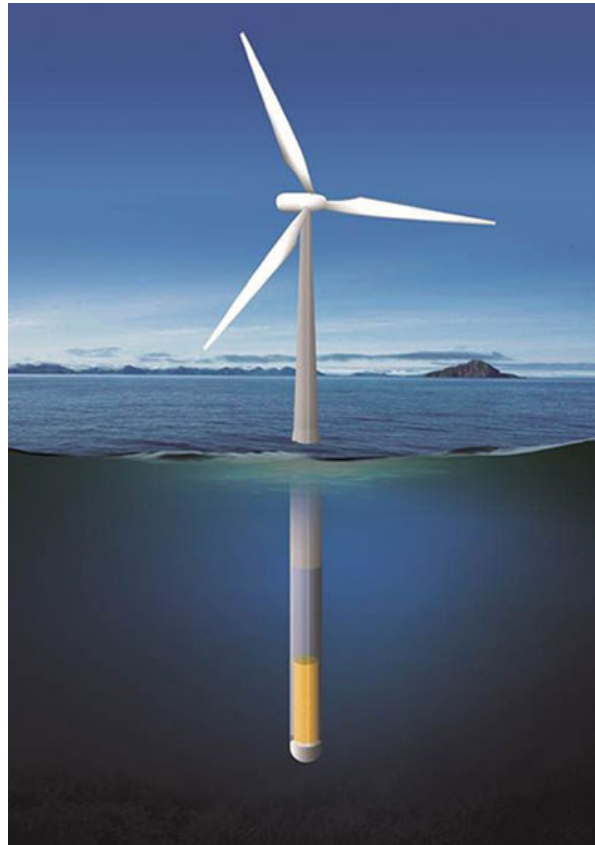
Figure 2.4: WindCrete monolithic design with residual compounds as ballast [13]
