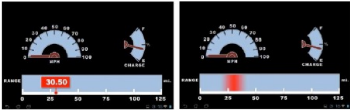
Figure 4: Remaining range was displayed as either highly precise values (left) or a diffuse color band (right) (Courtesy of Malte Jung).
