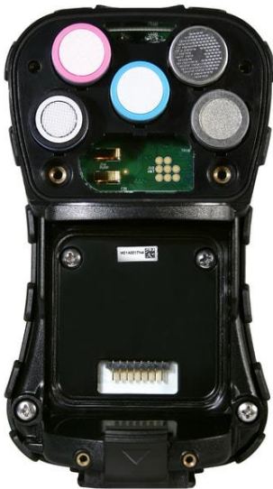
Figure 4-5: View on the inside of the Multi Rae Lite sensors (source: norrscope.com/product/multirae-sensors-accessories-spares )[58].
