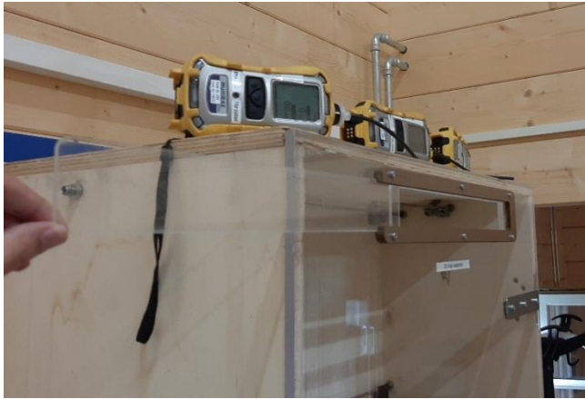
Figure 5-11: The ventilation grilles are manually opened in the case of open ventilation.
