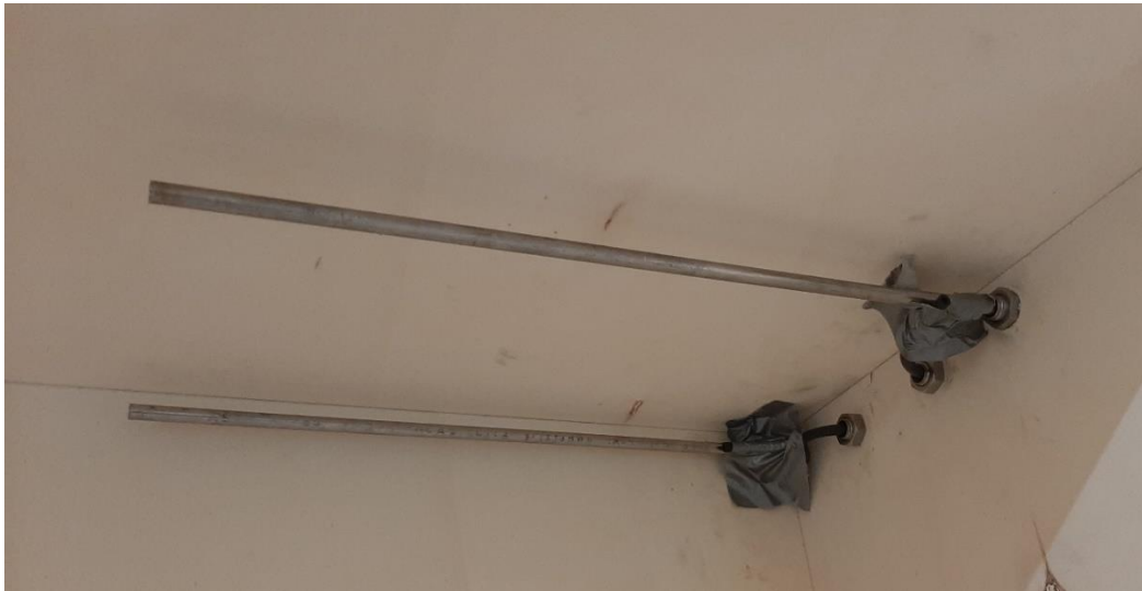
Figure 4-7: The sensor inlets of the four top sensors were positioned with the use of the metal and flexible tubes.
