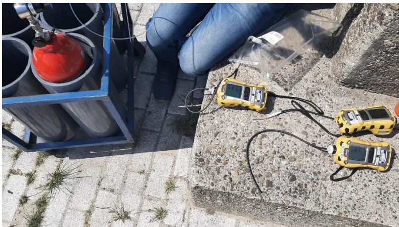
Figure 4-4: A bottle of hydrogen with test gas with the exact amount of 0.3 vol% hydrogen in Nitrogen. A Tedlar bag which can contain 5 liters of gas was used fill with test gas and was attached to the inlet of the sensors.
