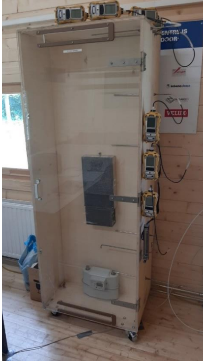
Figure 4-2: The test-setup with the sensors positioned at the top below the ceiling and on the side of the metering cabinet.
