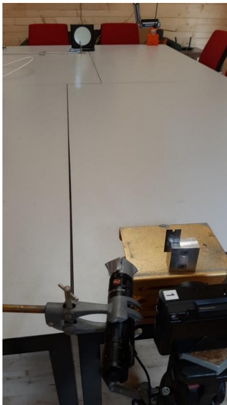
Figure E2: (a) Schlieren technique experimental set-up seen from the camera. (b) The outflow nozzle of hydrogen gas and the mirror in position on the other end of the table.
