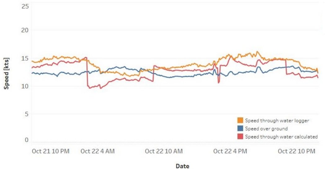
Figure 4.60: Speed through water and speed over ground for Slotergacht
