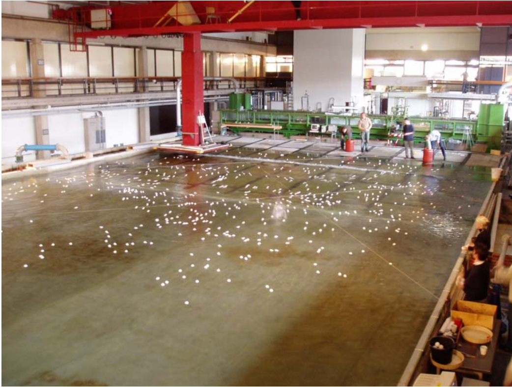
Figure 4-16: Seeding the recording area in the wave basin with floats
