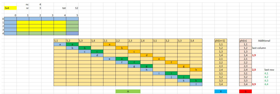
Figure 2.23: 3x4 test domain and its system of equations
