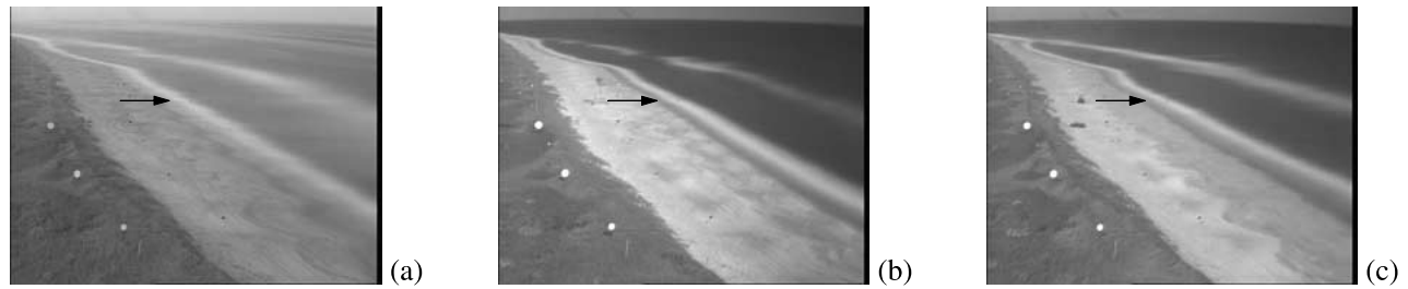
Figure 4. Time exposure video images showing Duck94 morphology on (a) 26 September 2100 UT ( \bar{t} \approx 268.5 days), (b) 30 September 1500 UT ( \bar{t} \approx 272.5 days), and (c) 4 October 1800 UT ( \bar{t} \approx 276.5 days). The arrows indicate the approximate alongshore location of the main cross-shore instrument array [Gallagher et al. , 1998]. The seaward white band, resulting from preferred wave breaking, indicates the approximate position of the sandbar. Ruessink et al. 's [2001] findings of alongshore uniformity in the sandbar [Ruessink et al. , 2001, Figure 9] were based on bathymetric surveys collected in a 350 m wide alongshore region centered around the main array, excluding the steep beach face.
