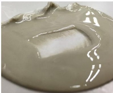
Figure 57: Filter cake – 20-25 \mu\text{m} filter with no additional particles at 0.25 bar
