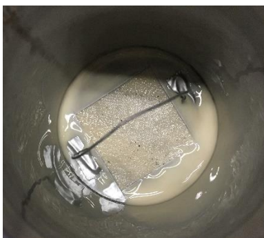
Figure 60: Filter cake - 250 filter with no additional particles at 1 bar
