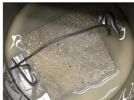
Figure 61: Filter cake - 250 filter with no additional particles at 1 bar close up
