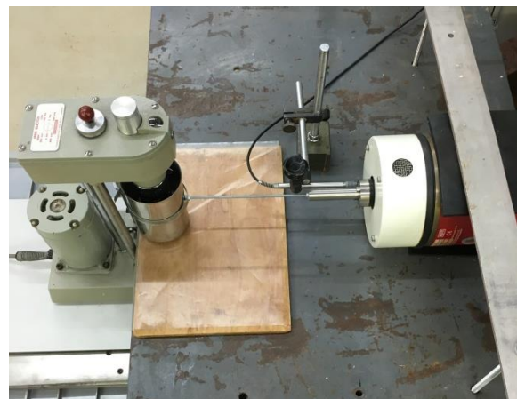
Figure 42: Horizontal vibration test setup top view
