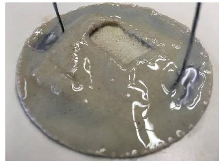
Figure 59: Filter cake – 250 \mu\text{m} filter with 9% 150-212 \mu\text{m} particles at 6 bar
