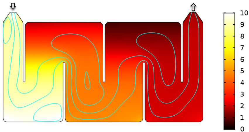
Figure 106: 2D simulation design 6 - Particle concentration [%] and stream lines
