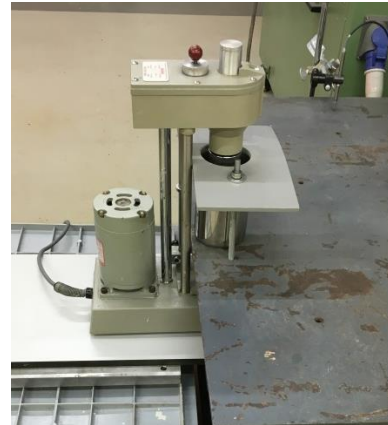
Figure 40: Vertical vibration test setup
