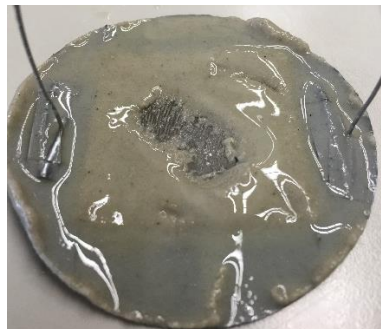
Figure 58: Filter cake – 63 \mu\text{m} filter with 17% 150-212 \mu\text{m} particles at 1 bar
