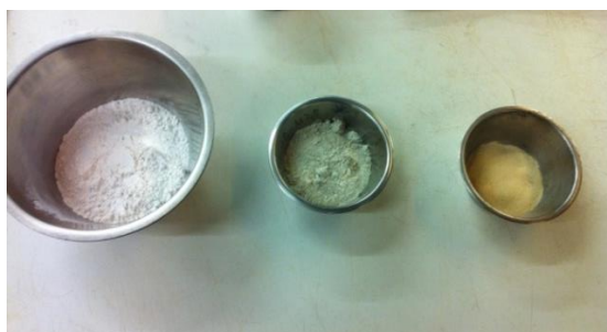
Figure 33: Drilling mud materials from left to right: Quarts flour, bentonite and Xanthan gum
