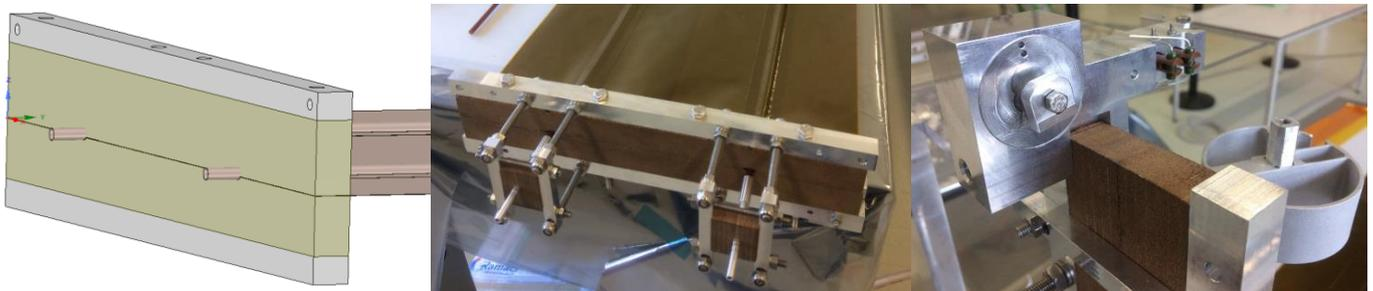
Figure 54: Foil Radiator Fixation 3D design to breadboard model and mounting of HDRM onto FRF
