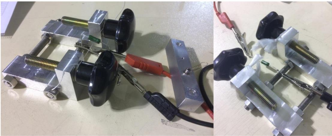
Figure 79: Dyneema thread thermal knife cutting tests
