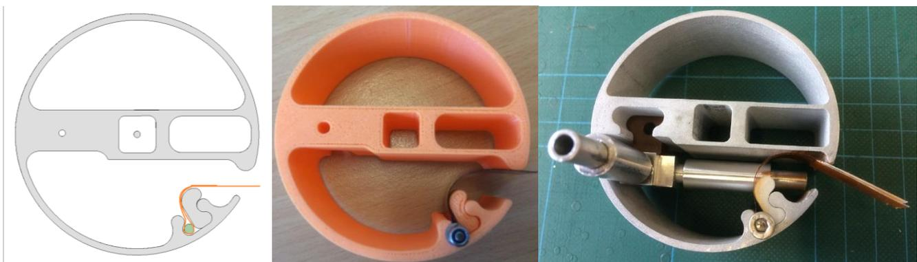
Figure 52: Roller: 3D CAD design, to 3d printed prototype, to 3d printed breadboard model
