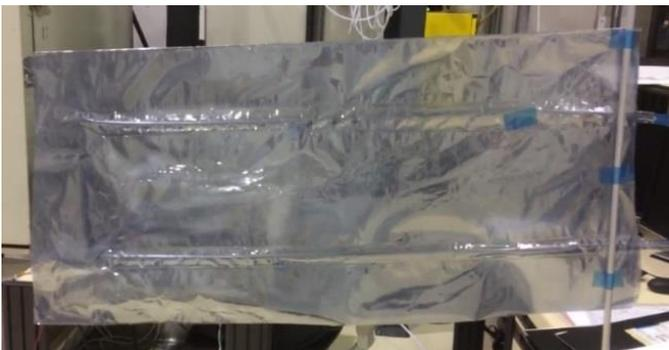
Figure 26: FR breadboard model made from PET/PE and pressurized with air at one bar pressure gauge
