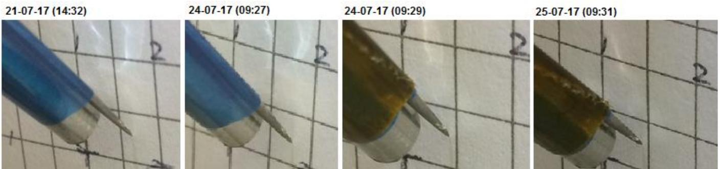
Figure 22: Creep test observations during various dates and times
