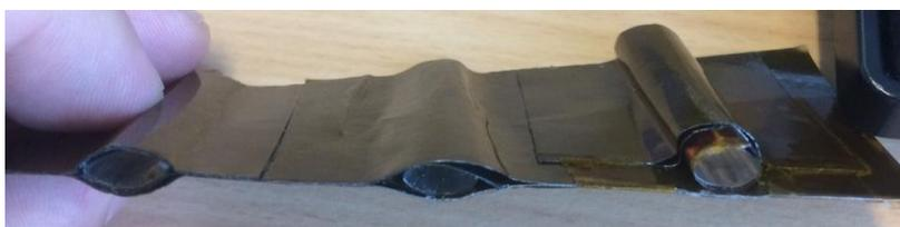
Figure 41: Tubing-laminate interfaces
