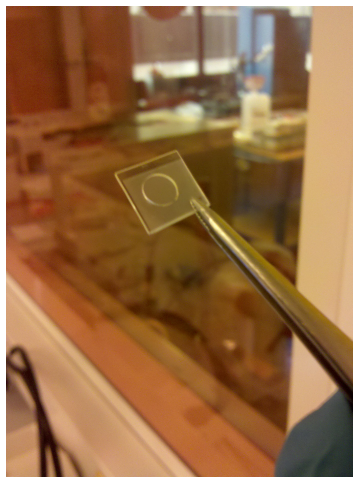
Figure F-1: Membrane on PDMS carrier used for migration and cell attatchement experiments.
