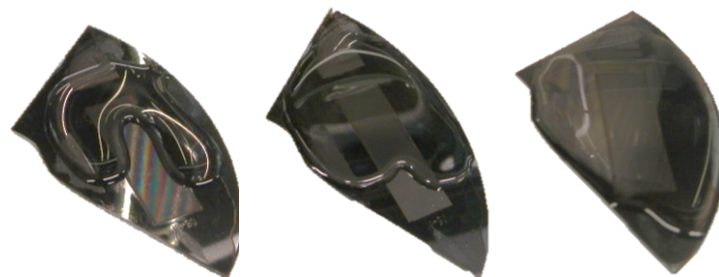
Figure A-4: (left) An uncured, degassed, 10:1 PDMS mixture is poured on an area of the mold containing no features. (middle & right) PDMS is left to flow to achieve complete coverage of the full array with features. This prevents formation of air traps.
